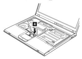
4. Secure the keyboard bezel from the underside of the computer with the screws **b** and **c**.
