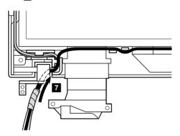
Move the spiral tube until it reaches at the cable guide of the LCD cover as in this figure. Make sure that the antenna cable is not pinched by cable clip ( a ).
