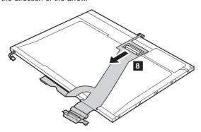
When installing: Make sure that the FPC connector is firmly attached to the LCD panel.
