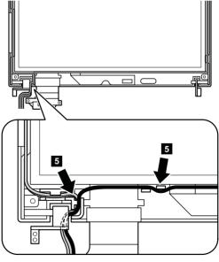
d. Coil the spiral tube round the antenna cables.
