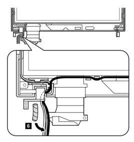
Slide the spiral tube in the direction shown by e. arrow 7.
