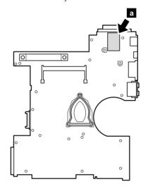
System board without the security chip (bottom view)
