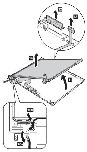
Remove the antenna assembly **a** and hinges **b** from the LCD assembly.
