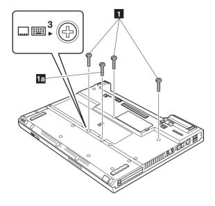
Note: Screw la is only for the models with 14.1-in. LCD. Other models do not have this screw.
