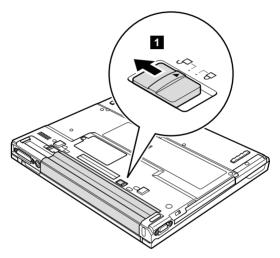
Holding the battery release lever in the unlocked position 2, remove the battery pack 3.
