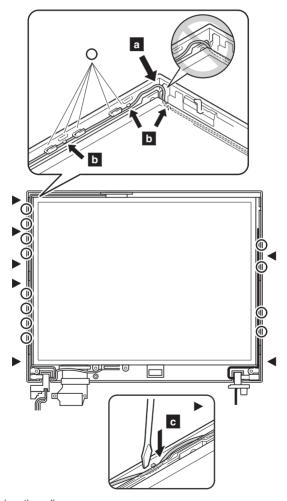
Then route the cables to along the cable guides of the LCD cover. When you route the cables around the LCD hinges, do as shown in **C**.
