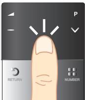
Press the ●●●●● button in the bottom centre of the Touch Pad. You can select a desired function (e.g. Menu(■), Source(⇨), Info(ℹ), etc.) easily.
