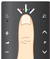
To display the colour button, exit button and play control buttons on the top of the screen, press the ●●●●● button on the top of the Touch Pad.
