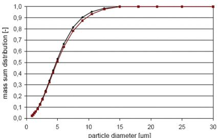
All measurements were obtained with a sodium chloride solution using a laser diffraction method. This diagram may not be applicable for suspensions or highly viscous medicines. More information can be obtained from the relevant medicine manufacturer.
