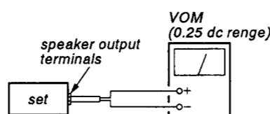
Adjust RT401 (L-CH) and RT451 (R-CH) for 0 V reading on the VOM.
