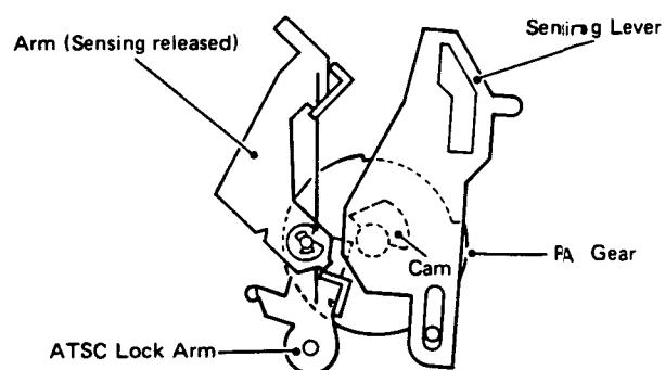
Fig. 22 At the time of PLAY (Sensing operation)
