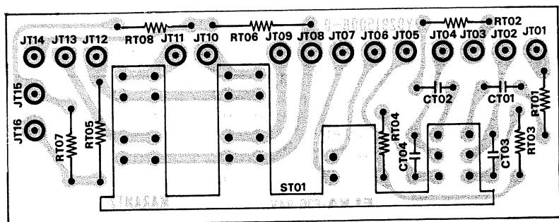
**Figure 15. Main Remote Assembly PT01 Component Locations**
