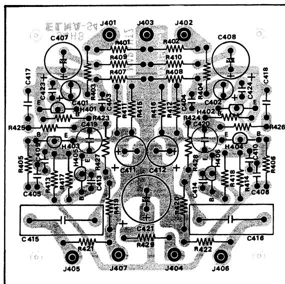
**Figure 9. Phono Amplifier Assembly P400 Component Locations**
