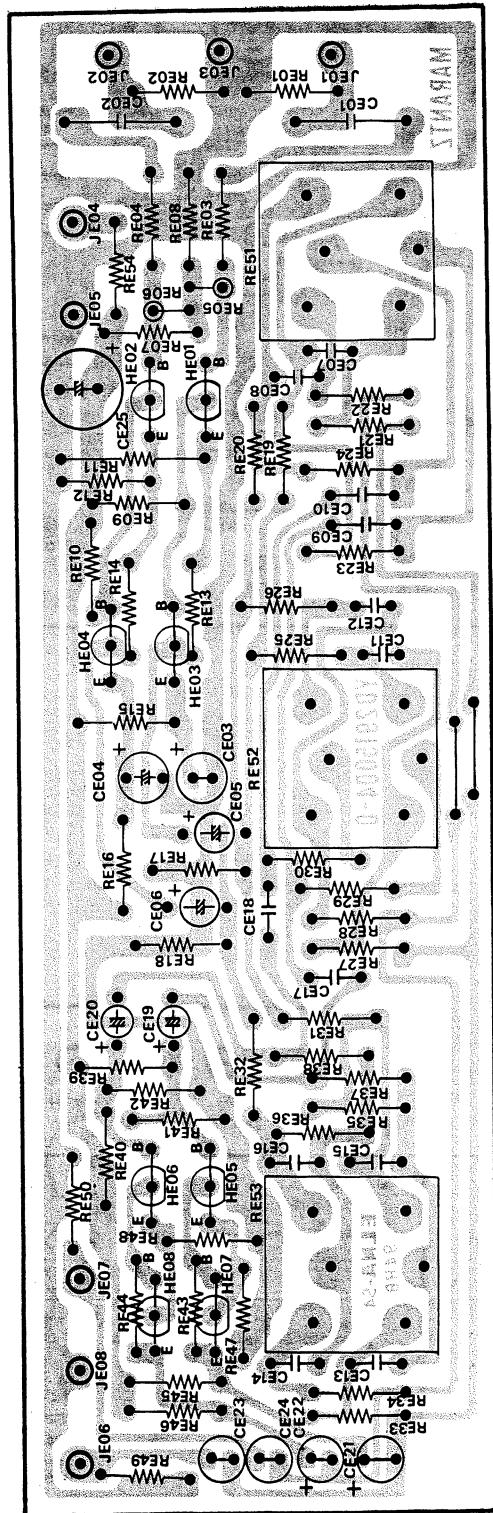
Figure 13. Tone Amplifier Assembly P500 Component Locations
