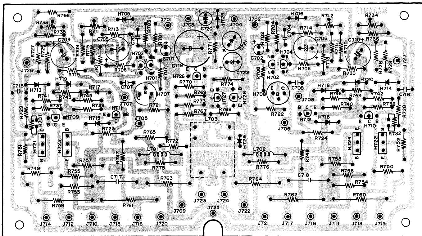
**Figure 10. Power Amplifier Assembly P700 Component Locations**
