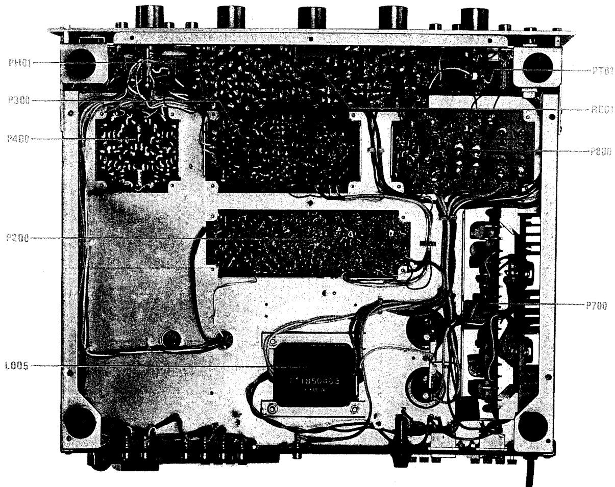
Figure 5. Main Chassis Component Locations (Bottom View)
