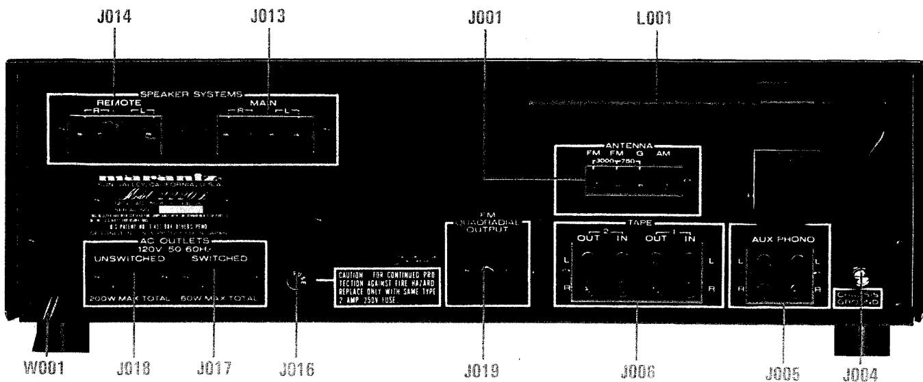
Figure 4. Rear Panel Adjustment and Component Locations
