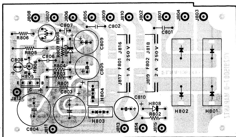
**Figure 11. Power Supply Assembly P800 Component Locations**
