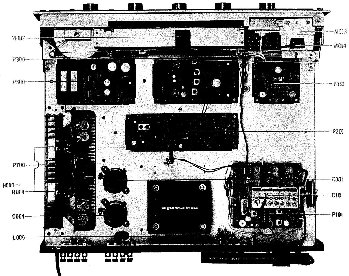
Figure 3. Main Chassis Component Locations (Top View)
