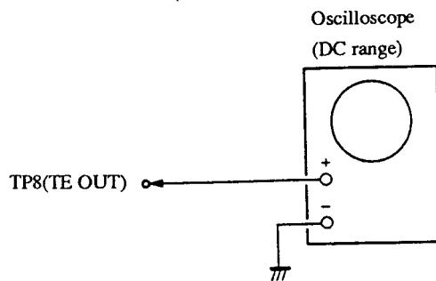
1. Keep the set horizontal. (If the set is not kept horizontally, this adjustment cannot be performed due to the gravity against the 2-axis device.)
