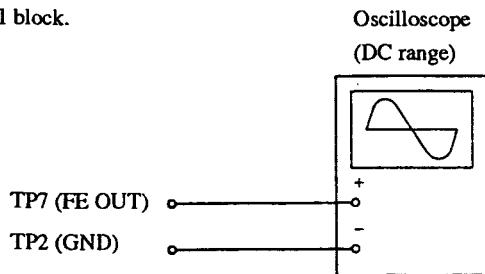
1. Connect an oscilloscope to test points TP7 (FE OUT) and TP2 (GND).
