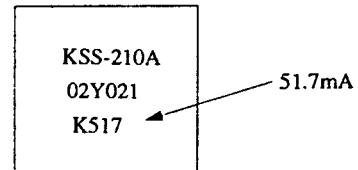
$$\text{Laser current } I_{op} = \frac{\text{Voltage across R4}}{10\Omega}$$
