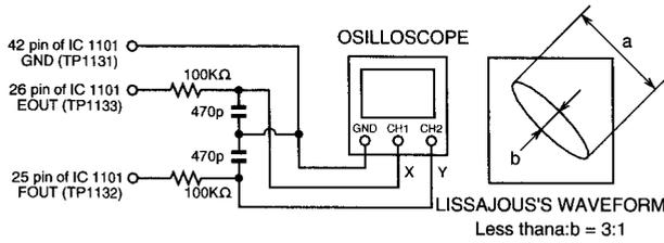
**Figure 23-1 Optical Pickup Grating Deviation Measuring Method**
