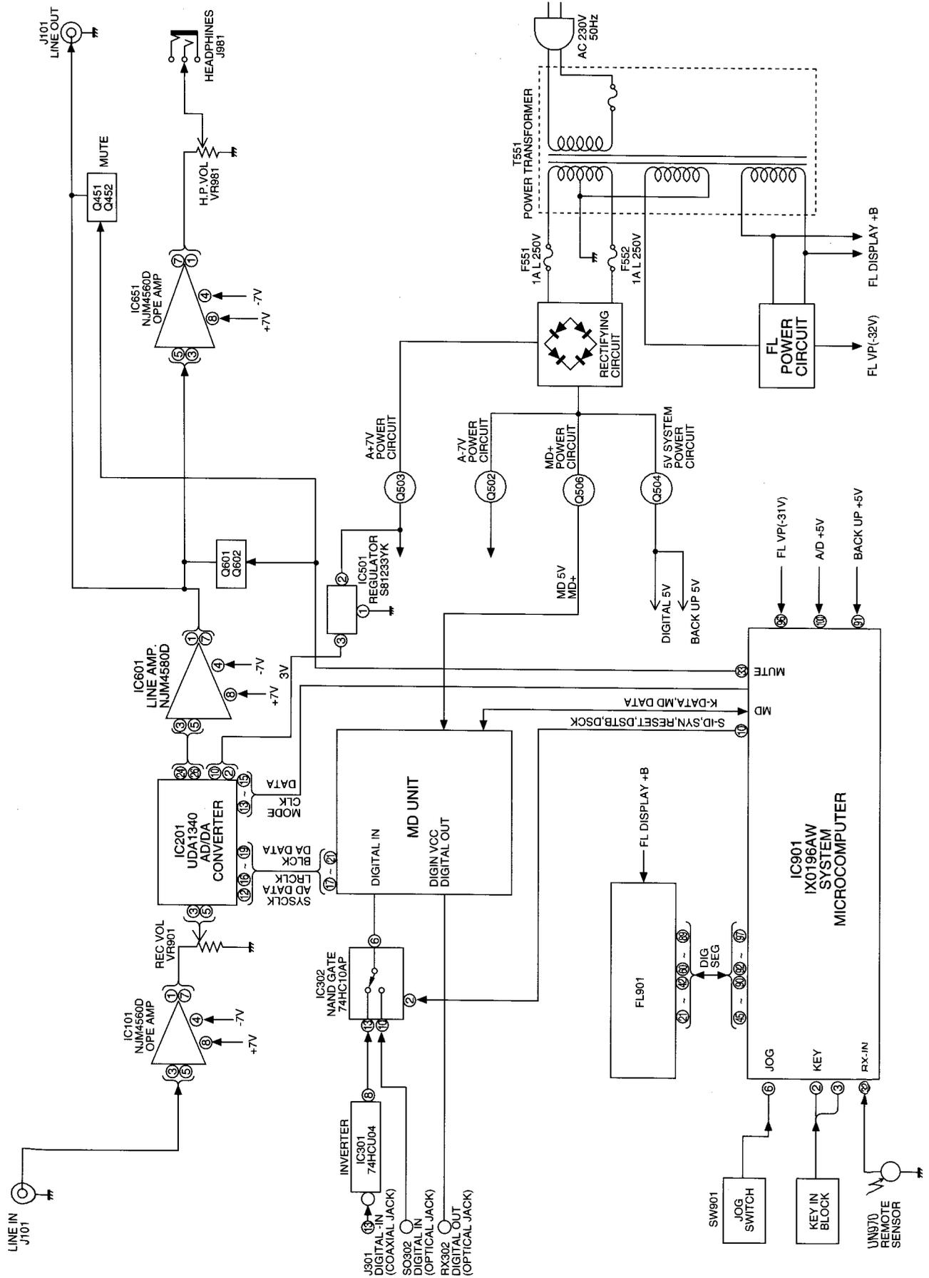
Figure 29 BLOCK DIAGRAM (2/2)
