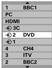
HDMI displays equipment connected to *Input HDMI* on the back of the television. It is designed for best performance with 1080i high definition signals.
